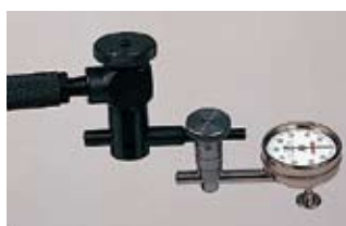
Far Left: 651B1 Indicator gripped directly to its stem via the post snug
